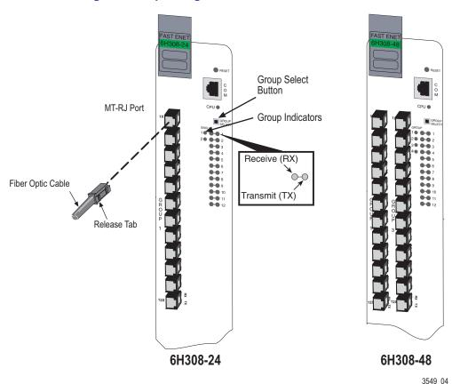
Figure 3-3 Connecting a Fiber Optic Segment to the Module
